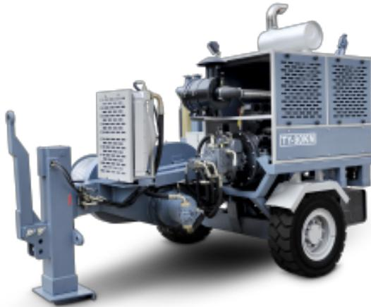
This machine allows for the tension stringing of twin-bundle conductor of 500mm<sup>2</sup> and below in mountainous and hilly areas, of twin-bundle conductor of 630mm<sup>2</sup> and below in flat lands, and of single conductor 720mm<sup>2</sup> in various terrains; besides, it can be used for traction stringing of OPGW or ADSS optical cable and 220kV haulage rope in various terrains.
